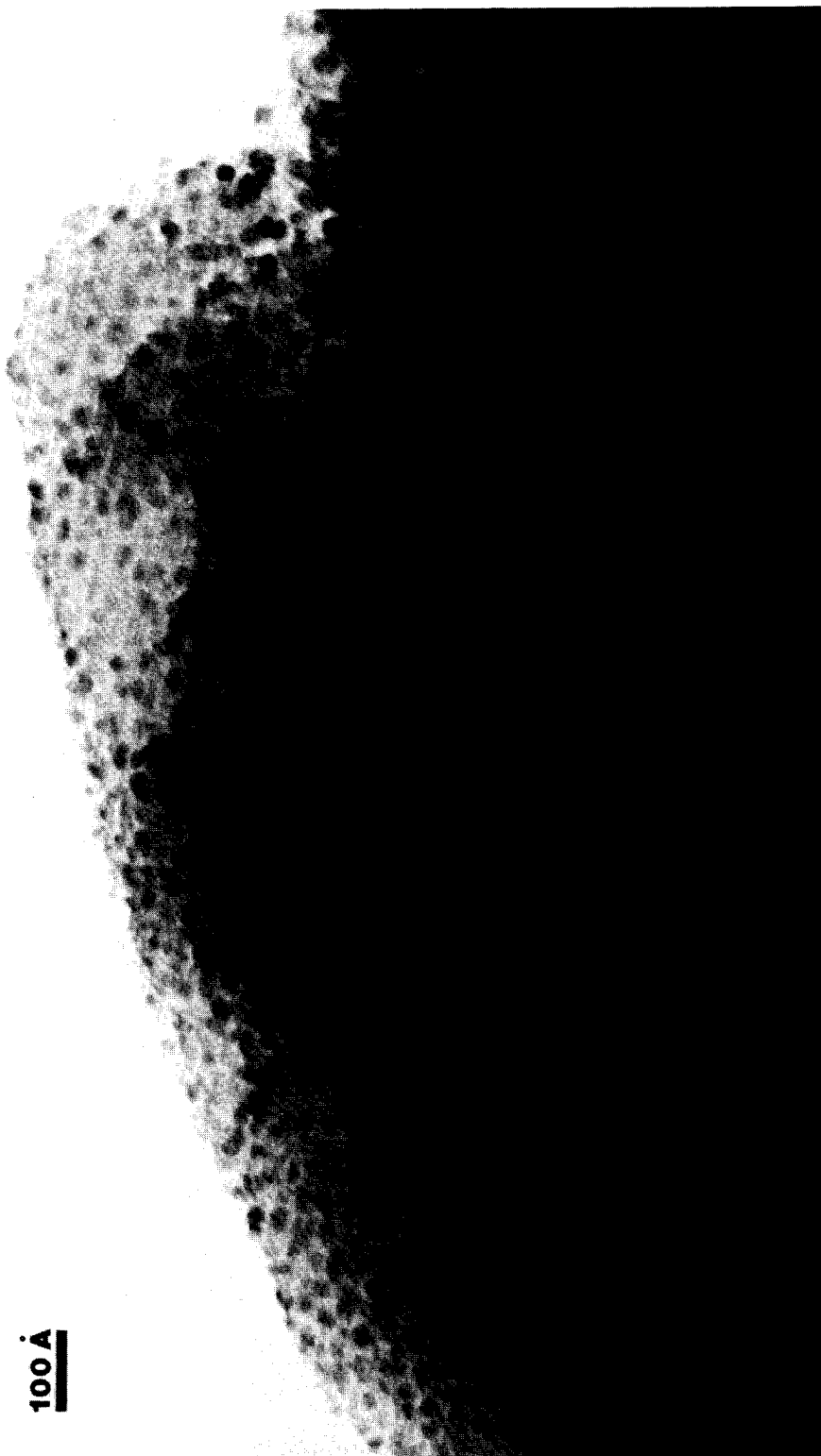
FIG. 3. Transmission electron micrograph of Rh-ZK-5 (3.5% Rh).
